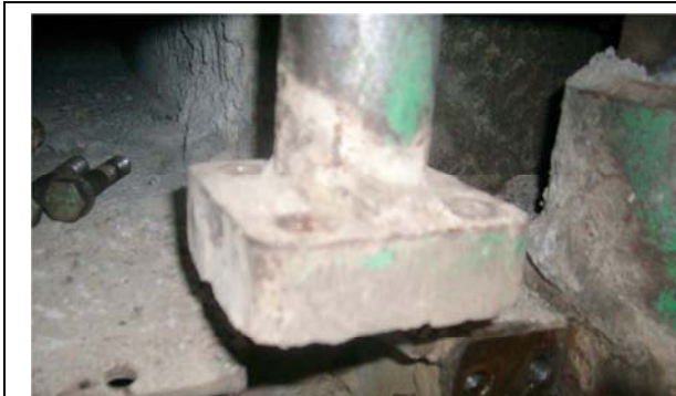
Shaker shaft and hold down collar are covered in material which with the damages to the vibrator you would also have damages to the shaker shaft button on the bottom. Because of these damages the shaker shaft must be replaced.
