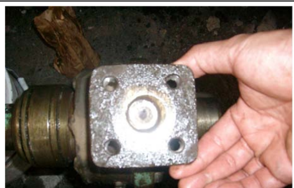
Damages to eccentric foot are evidence the bolts had backed off allowing the shaker shaft to hammer and eventually breaking the bolts.
